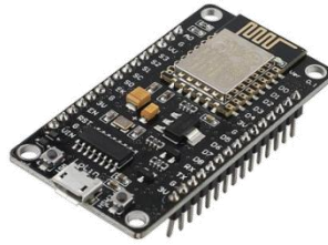
Figure 4: NodeMcu module in combination with CH340G chip
