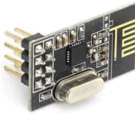
Figure 9: NRF24L01 + wireless transmitter and receiver module
