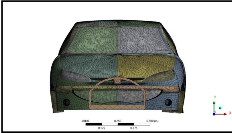
Figure 5. The meshing of the analyzed car
