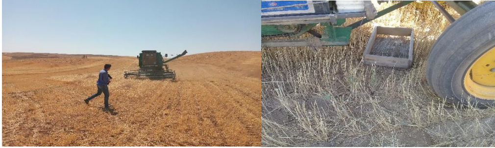
Figure 4: How to install the wooden and metal frame in the center of the rear wheels of the combine perpendicular to the direction of motion
