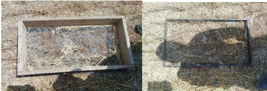
Figure 5: Wooden frame of the end of the combine loss- the metal frame of the John Deere 1055i combines platform
